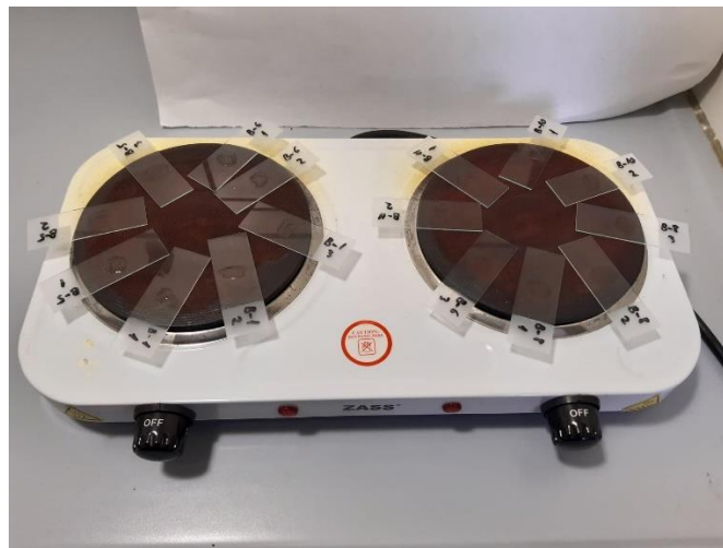
Fig. 3. Burning the slides with the diatom samples on the electric hob
